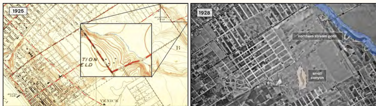
Figure 4. A 1925 USGS topographic map depicts SMO's ephemeral stream as a dotted blue (left). Aerial photograph (C-300 J-286) from a 1/1/1928 flight shows erosion and vegetation along the stream path, highlighted in blue (right).
